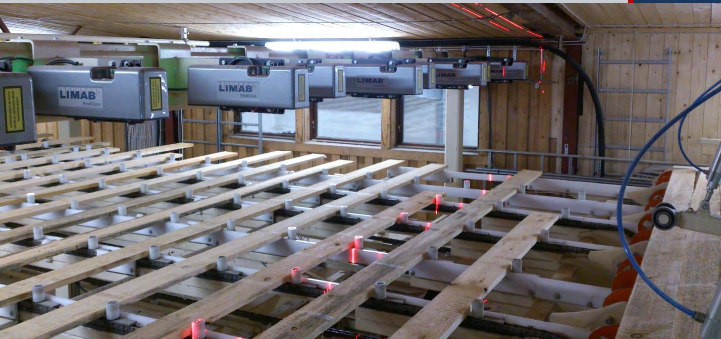
Laser based board scanning with high resolution
