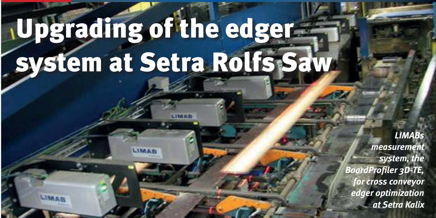
*LIMABs measurement system, the BoardProfiler 3D-TE, for cross conveyor edger optimization at Setra Kalix*
