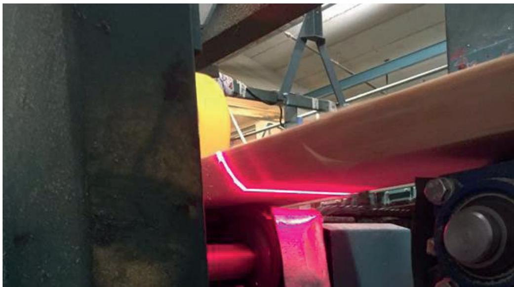
*LIMABs measurement system, the BoardProfiler 3D-LE, for lineal conveyor edger optimization*
